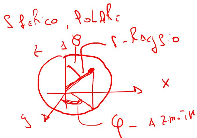
$$\nabla f(r, \theta, \phi) = \frac{\partial f}{\partial r} \hat{e}_r + \frac{1}{r} \frac{\partial f}{\partial \theta} \hat{e}_\theta + \frac{1}{r \sin \theta} \frac{\partial f}{\partial \phi} \hat{e}_\phi$$
